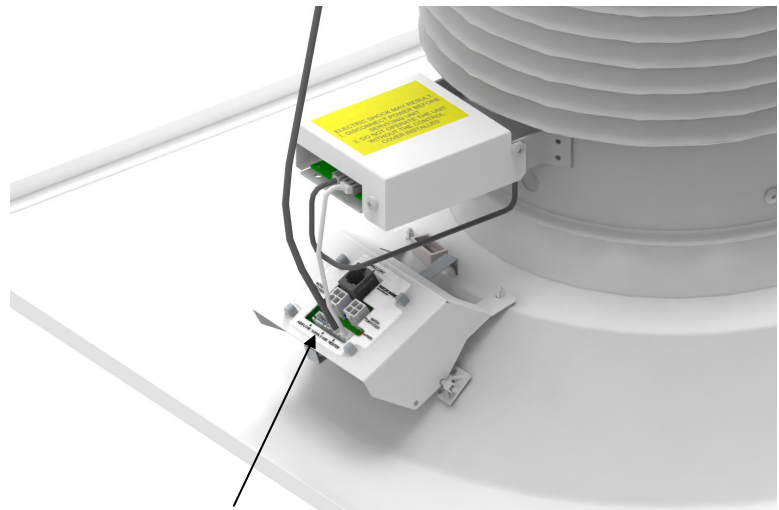
Plug the change-over sensor into this connector on activated masters only.
