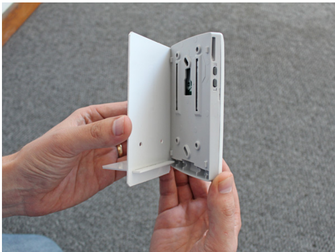
Insert the short tongue of the Foot-plate into the slot in the bottom of the thermostat.
