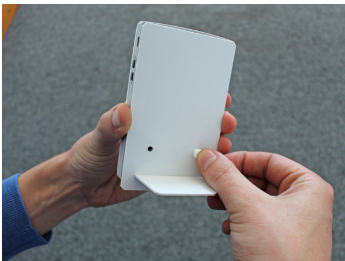
Align the holes in the stand with the holes in the thermostat and push the 2 plastic rivets all the way home.
